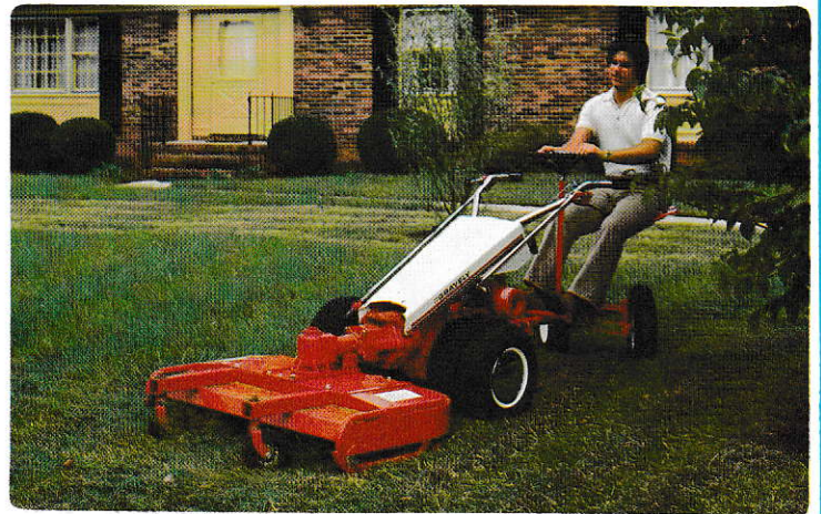
Gravelly 524 Convertible Tractor with optional Steering Sulky. Sulky must be used with optional Dual Wheels.
