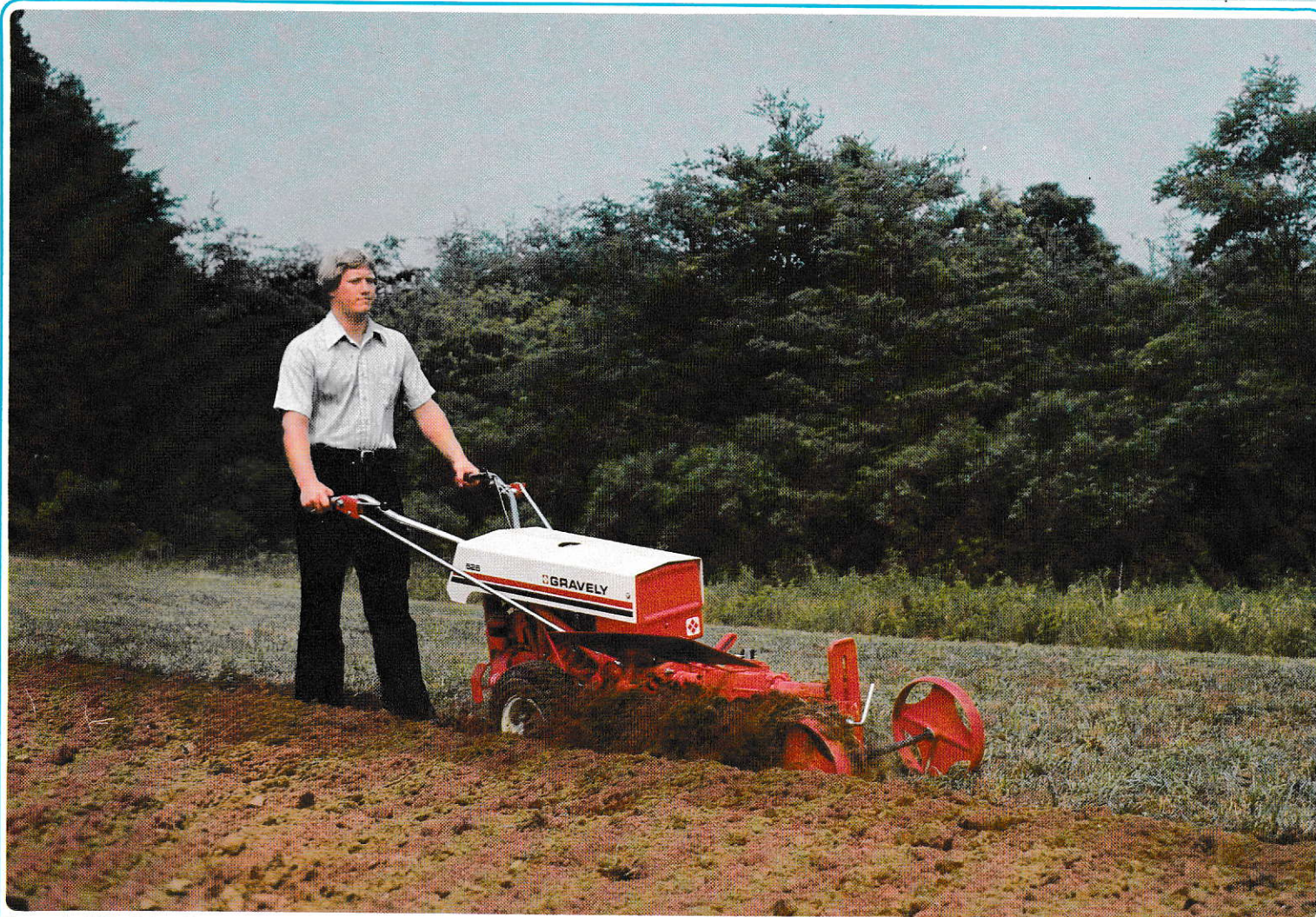
Gravely 526, 8 hp Convertible Tractor with famous all-gear-drive Rotary Plow.
