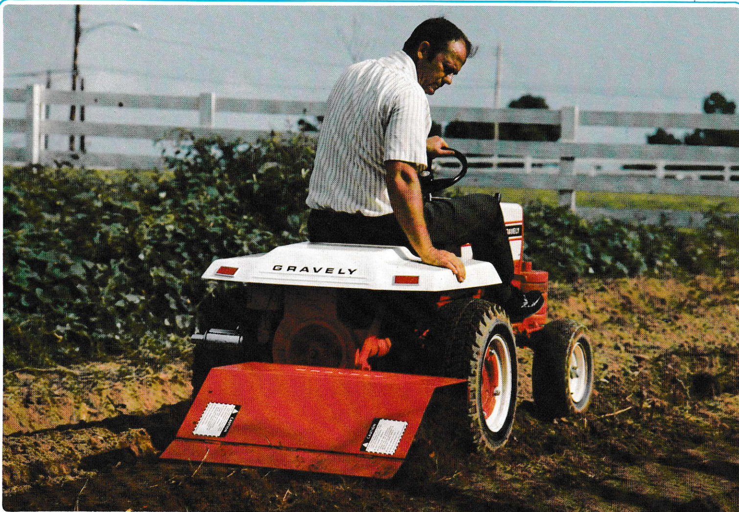
Gravely 816S, 16 hp Riding tractor with all-gear drive Rear Tiller, optional front Weight Rack w/Weights and opt. Rear Wheel Weights
