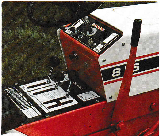
One-lever instant forward-neutral-reverse
