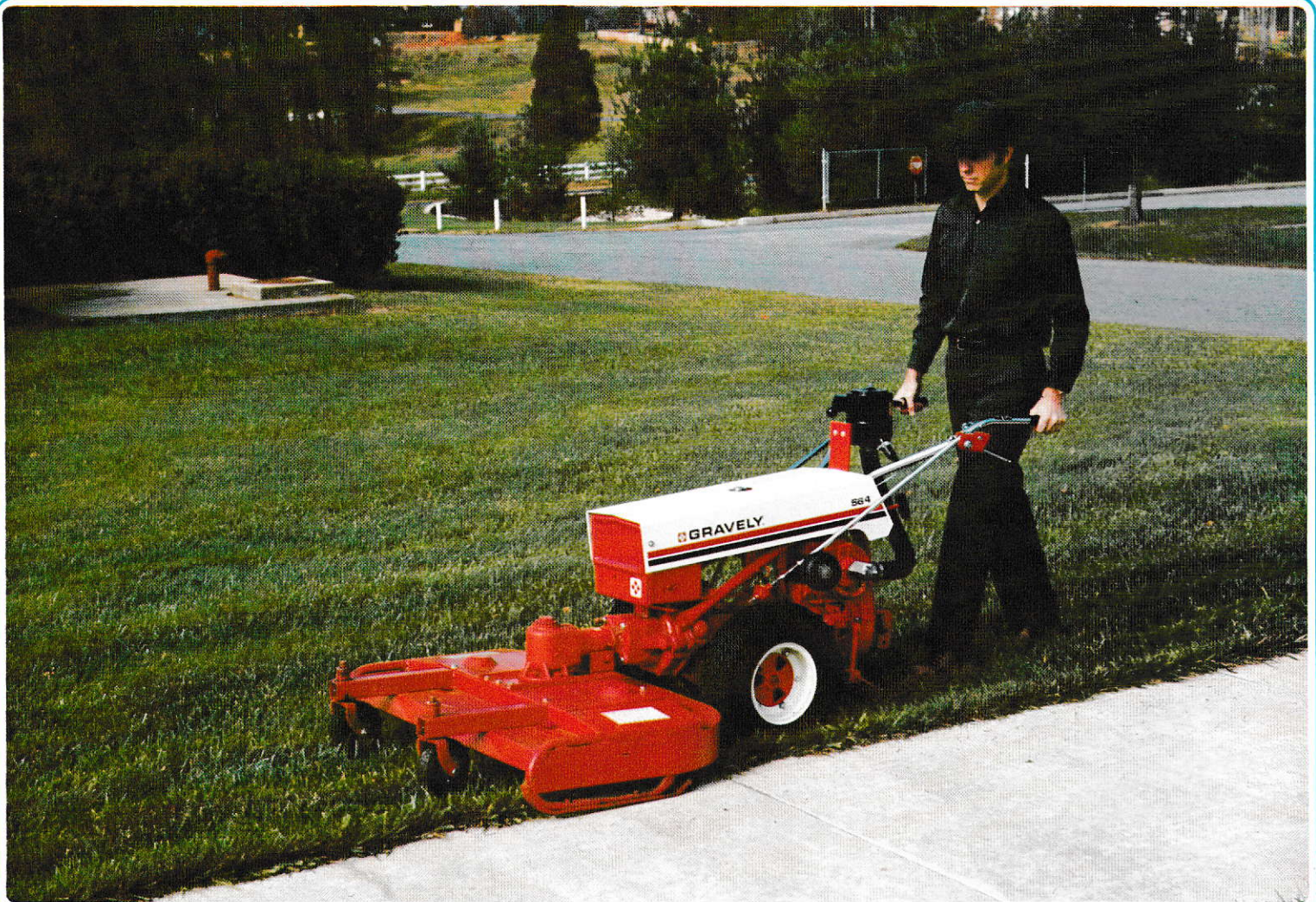
Gravely 564, 12 hp Commercial Convertible Tractor, manual start with 40-inch Commercial Rotary Mower
