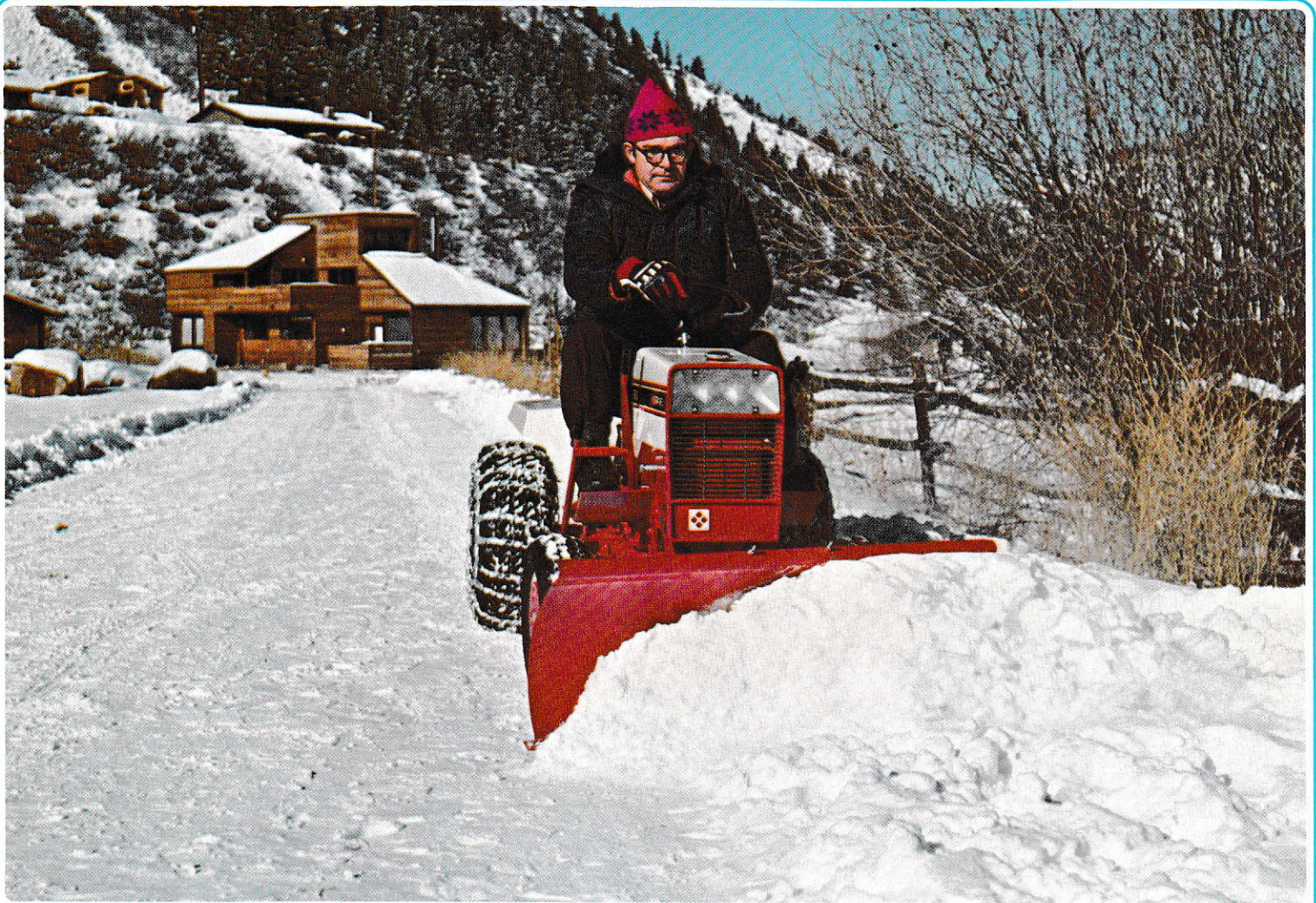
Gravely 812, 12 hp Riding Tractor with 48-inch SnowDozer, optional Tire Chains and Wheel Weights.
