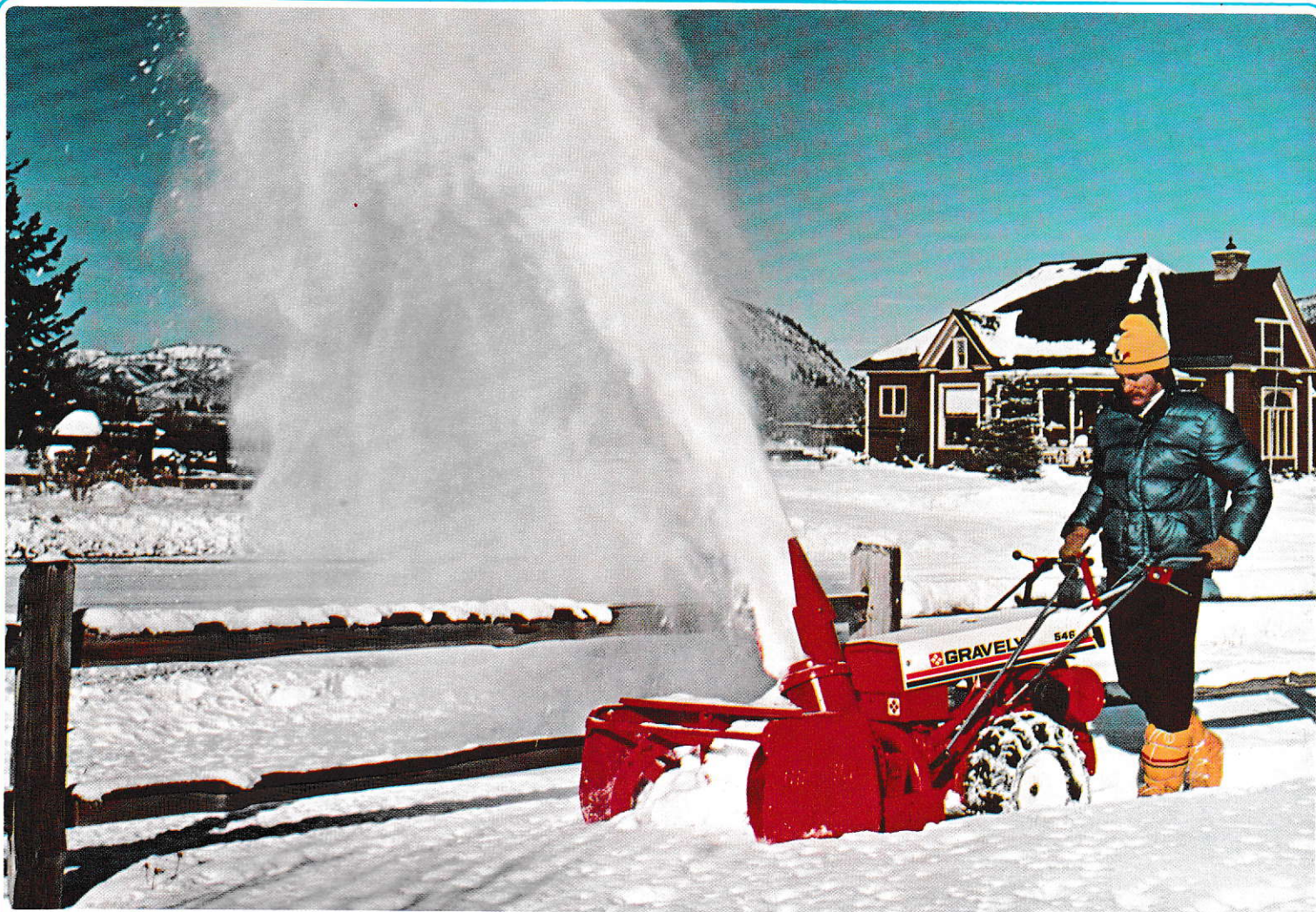
Gravelly 546, 10 hp Convertible Tractor with 34-inch Snowblower and optional Tire Chains.
