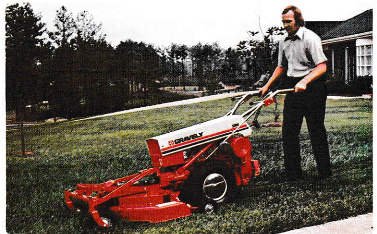
Gravely 566, 12 hp Convertible Tractor with 40-inch Rotary Mower and optional Chrome Wheel Covers
