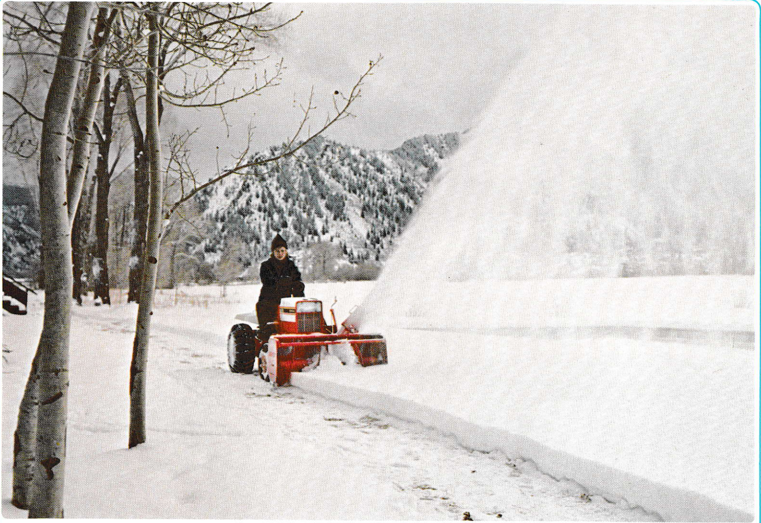
Gravelly 816S, 16 hp, 44-inch Snowblower: optional front and rear Wheel Weights, Tire Chains, Weight Rack Kit, plus Weights
