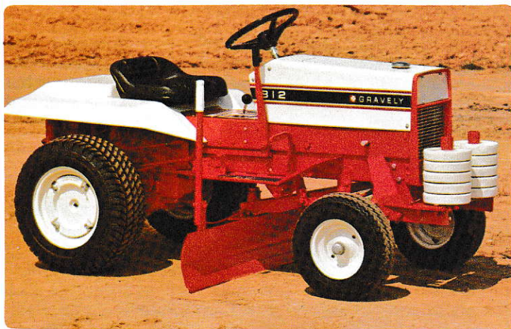
Gravely 812, 12 hp Riding Tractor with 48-inch Center-Mount Blade. Optional Front Weight Rack with Weights and optional Rear Wheel Weights.
