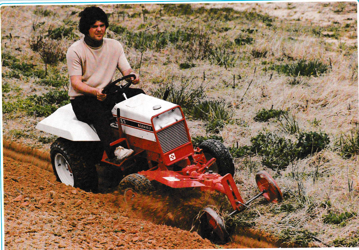
Gravelly 816S, 16 hp Riding Tractor with All-Gear-Drive Rotary Plow
