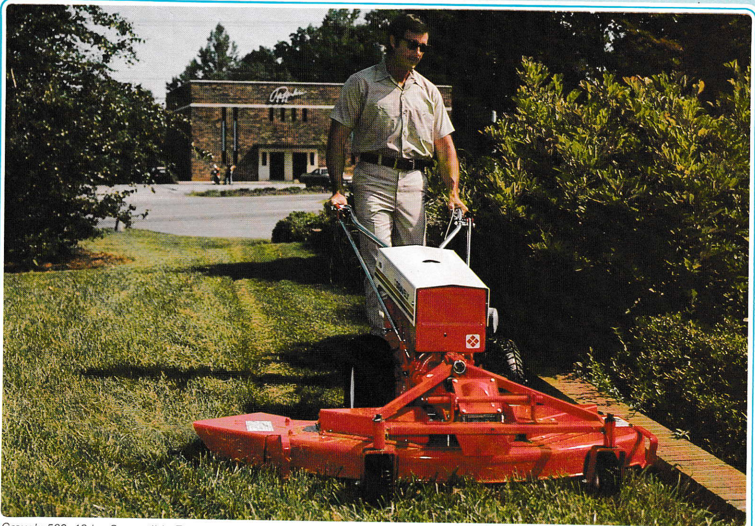
Gravelly 566, 12 hp Convertible Tractor with 50-inch Rotary Mower
