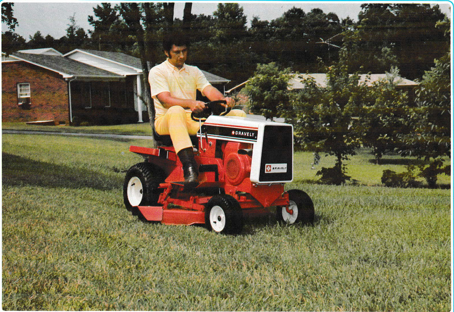
Gravely 8 hp, 408 Lawn Tractor with 34-inch Rotary Mower
